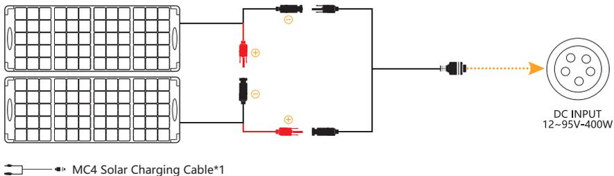
✘ It is recommended to choose PECRON solar panels for optimal user experience! The VOC of a single solar panel should be less than 95V, and the VMP should be greater than 6V.
