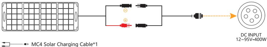
✘ It is recommended to choose PECRON solar panels for optimal user experience! The VOC of a single solar panel should be less than 95V, and the VMP should be greater than 12V.
