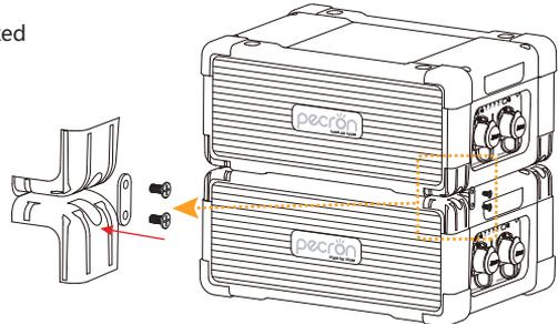
3: Install the protective corners in the following order: align the side with the positioning structure first, then snap the front side into place. Install them one by one until they are properly positioned.
